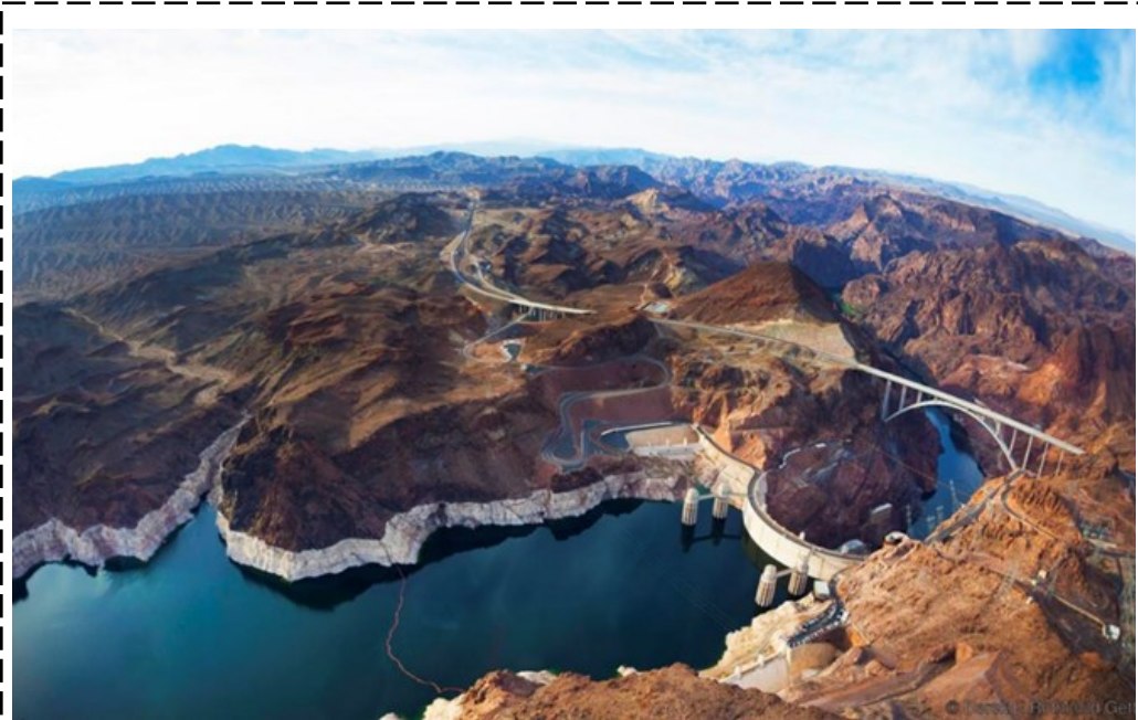
Pictured above: An aerial view of Lake Mead at Hoover Dam. From this view the drop in the water surface elevation is clearly indicated by the white ring around the perimeter of Lake Mead.
