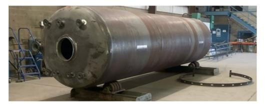
A new 5,000 gallon ASME certified pressure vessel is in the process of fabrication. This work is typical of the ongoing effort by the Water Utility to reinvest in the communities water system infrastructure.
