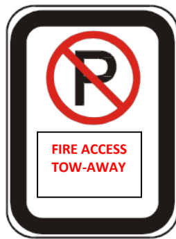
FIGURE D103.6 FIRE LANE SIGNS
