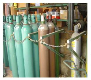
Cylinders, valves, regulators, hoses as well as other apparatus and fittings for oxygen shall be kept free from oil and grease. Oxygen cylinders, apparatus, and fittings shall not be handled with oily hands, oily gloves, greasy tools or equipment.
