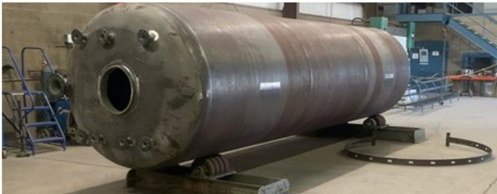
*A new 5,000 gallon ASME certified pressure vessel is in the process of fabrication. This work is typical of the ongoing effort by the Water Utility to reinvest in the communities water system infrastructure.*
